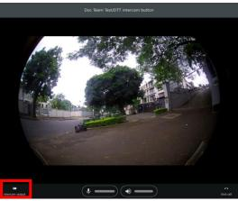
→ Click the intercom output button to toggle the relay output.
